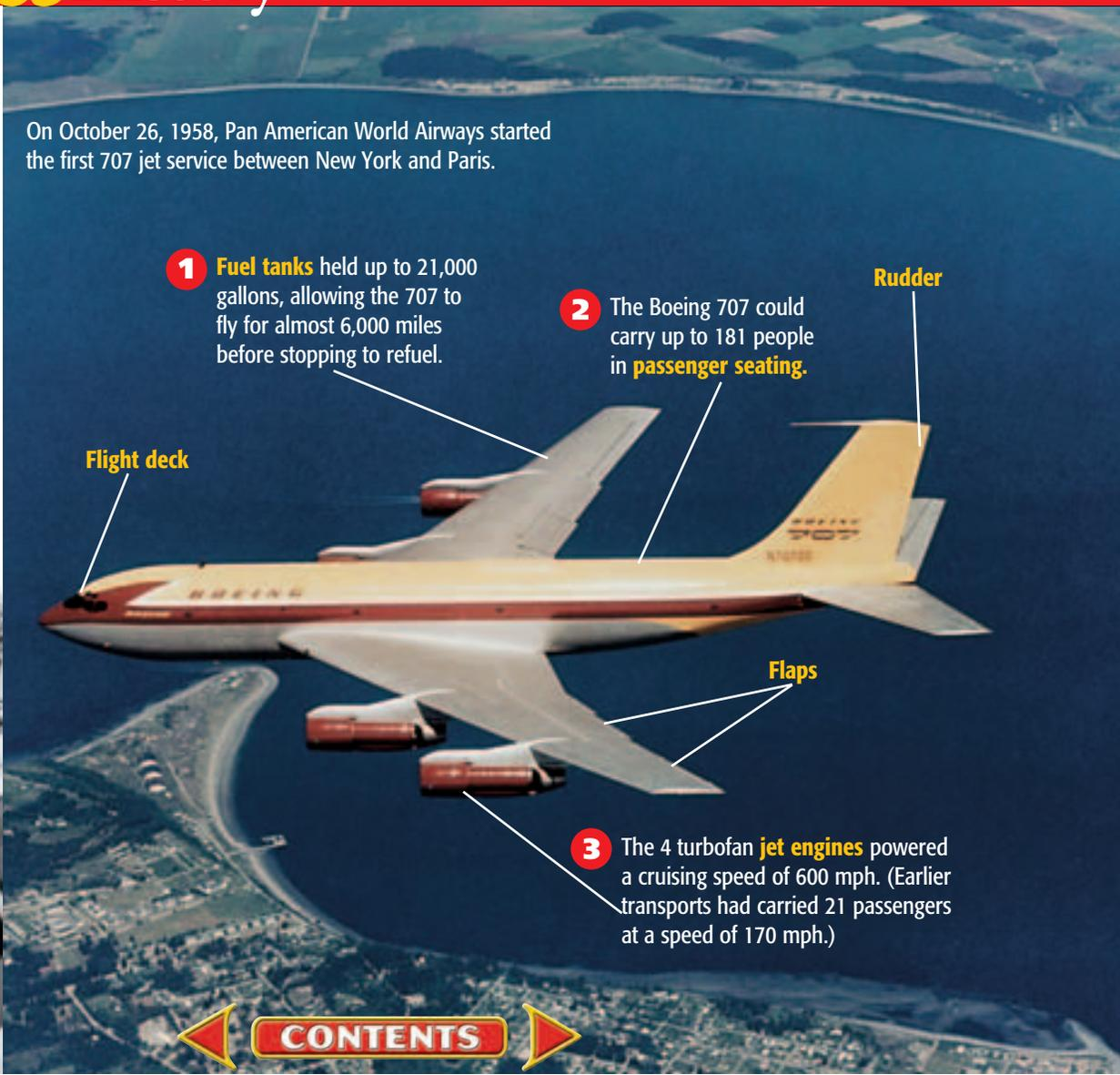
**1** **Fuel tanks** held up to 21,000 gallons, allowing the 707 to fly for almost 6,000 miles before stopping to refuel.
